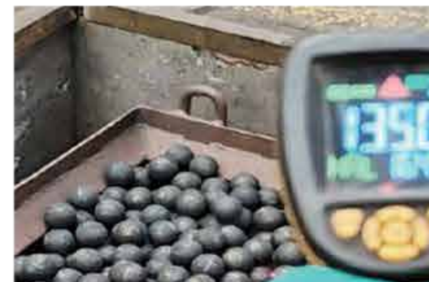
TEMPERATURE DETECTION DURING PRODUCTION
